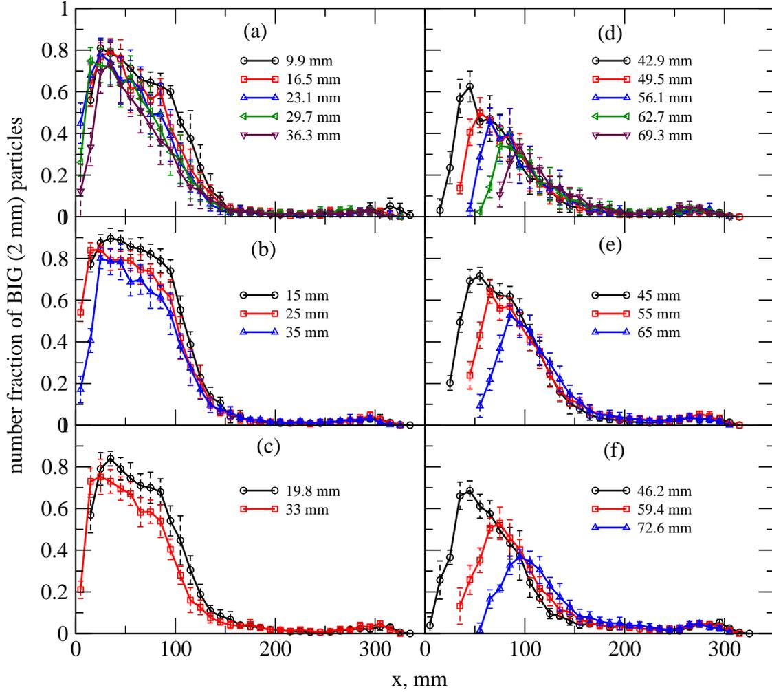
**Figure 3:** Profiles of number fraction of big (2 mm) particles along the flow direction,  $x$  (mm) across the depth in the flowing layer,  $y$  (mm), for equal % of mixture. Volume of pouring (a) 100 gm (b) 150 gm and (c) 200 gm for top region and similarly for bottom region (d), (e) and (f). Height of the divider from the bottom (h): 22 cm. Error bars show the standard deviation over eight experiments.
