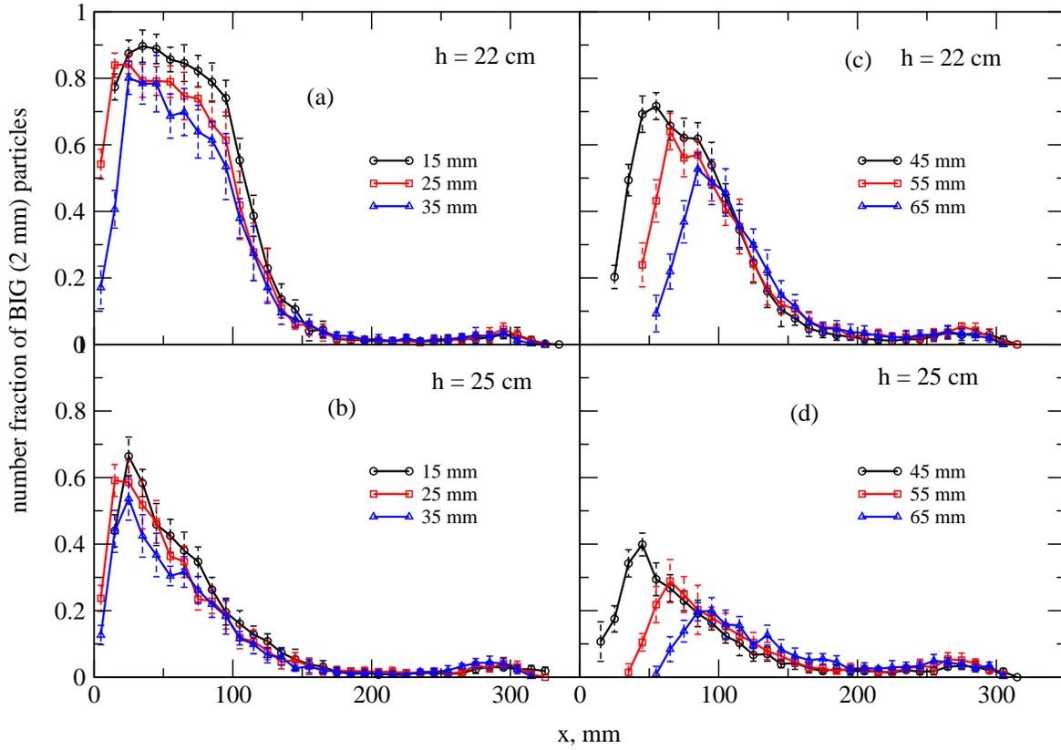
**Figure 4:** Profiles of number fraction of big (2 mm) particles along the flow direction,  $x$  (mm) across the depth in the flowing layer,  $y$  (mm) for equal % of mixture. Height of the divider from the bottom (a) 22 cm, and (b) 25 cm for top region and similarly for bottom region (c), and (d). Volume of pouring: 150 gm. Error bars show the standard deviation over eight experiments.
