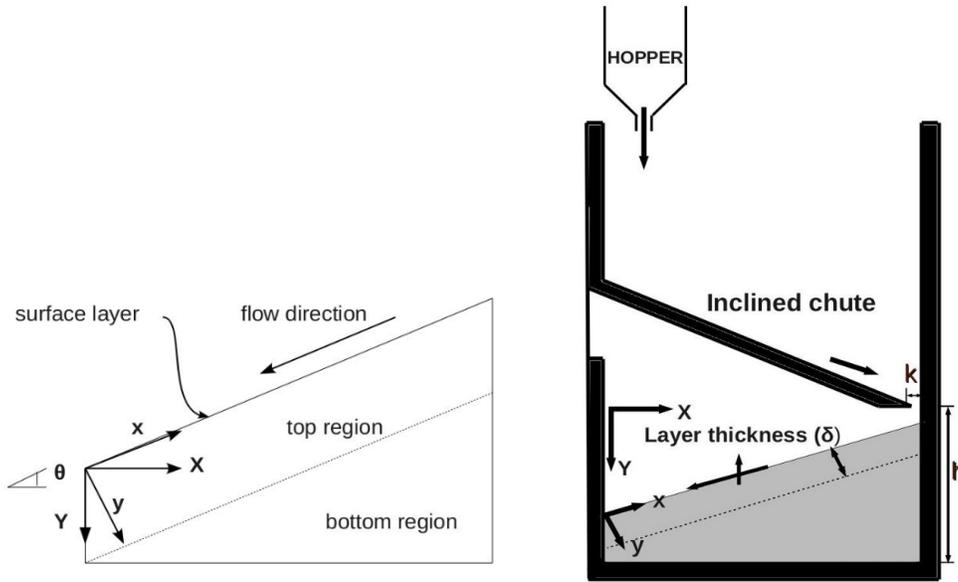
**Figure 1:** Schematic view of heap formation, comprising top and bottom region (left) along with setup used (right). Coordinate system shows  $x=0$ ,  $y=0$  at the low end of the top surface of the pile. The coordinate system employed in the analysis is shown (left).
