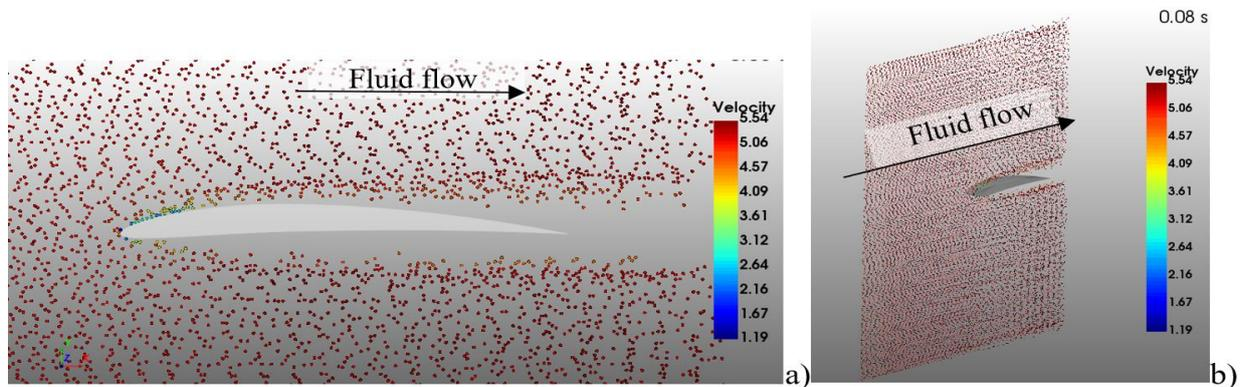
**Figure 4:** Flow around wing profile in particle contaminated media a) side view b) orthogonal view. Velocity is given in  $\text{m s}^{-1}$ .
