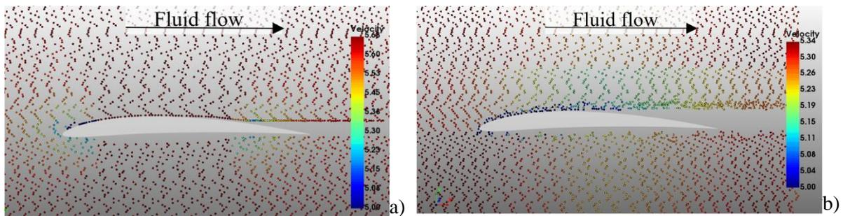
**Figure 5:** a) Flow around profile in  $\mu = 0.01 \text{ Pa s}$  viscosity media, translational velocity of particles are displayed, b) Flow around profile in  $\mu = 10 \text{ Pa s}$  viscosity media, translational velocity of particles are displayed. Velocity is given in  $\text{m s}^{-1}$ .
