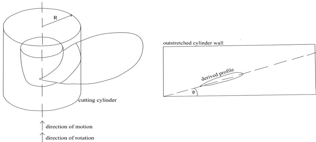
**Figure 2:** The derivation of the profile.  $R$  is the radius belonging to the derived profile.  $\phi$  is the pitch of the derived profile [10].
