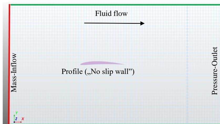
**Figure 3:** Computational area, Red zone: mass inflow. Green zone: pressure- and material-outlet. The dimensions of the domain are 0.6 m by 0.34 m.
