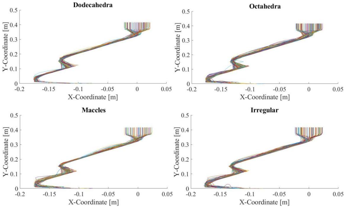
Figure 9: Trajectories for 10 carat diamonds grouped by particle shape for Design C.
