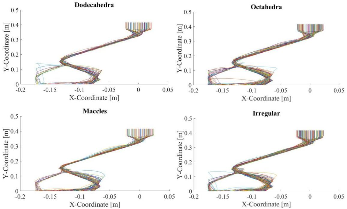
Figure 7: Trajectories for 10 carat diamonds grouped by particle shape for bin Design B.
