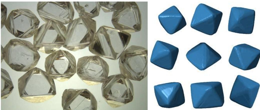
Figure 2: Examples of real octahedral diamonds vs high-fidelity images captured by the RhoVol machine.
