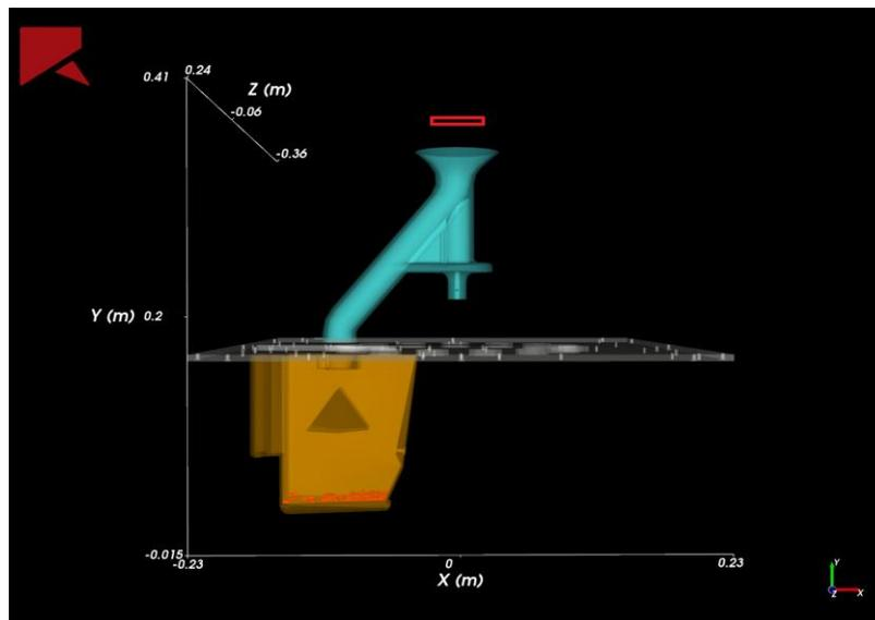
Figure 3: Simulation setup in Rocky. The particles are released (red square) into the sorting tube (blue) which directs them into the sorting bin (orange).
