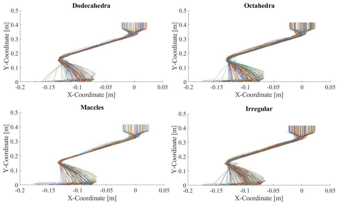
Figure 5: Trajectories for 10 carat diamonds grouped by particle shape for Design A.
