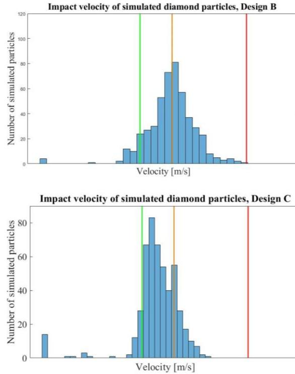
Figure 10: Maximum impact velocity distribution for 10 carat diamonds grouped by different bin designs.
