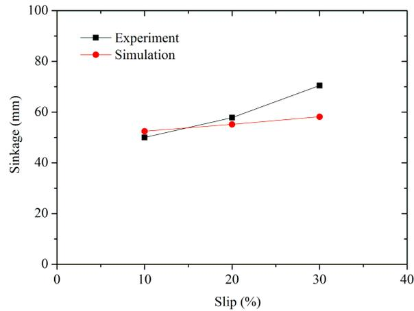
**Figure 8:** The rim sinkage versus the slip rate in the simulation
