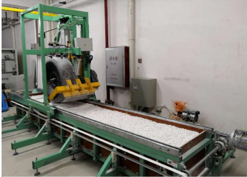
**Figure 3:** Soil bin test facility
