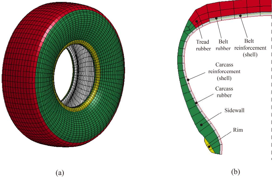
**Figure 4:** FE model of pneumatic tire: (a) tire model; (b) cross-sectional model
