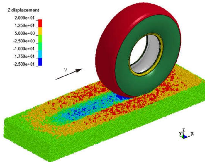
**Figure 6:** Z-displacement contour of the granular terrain
