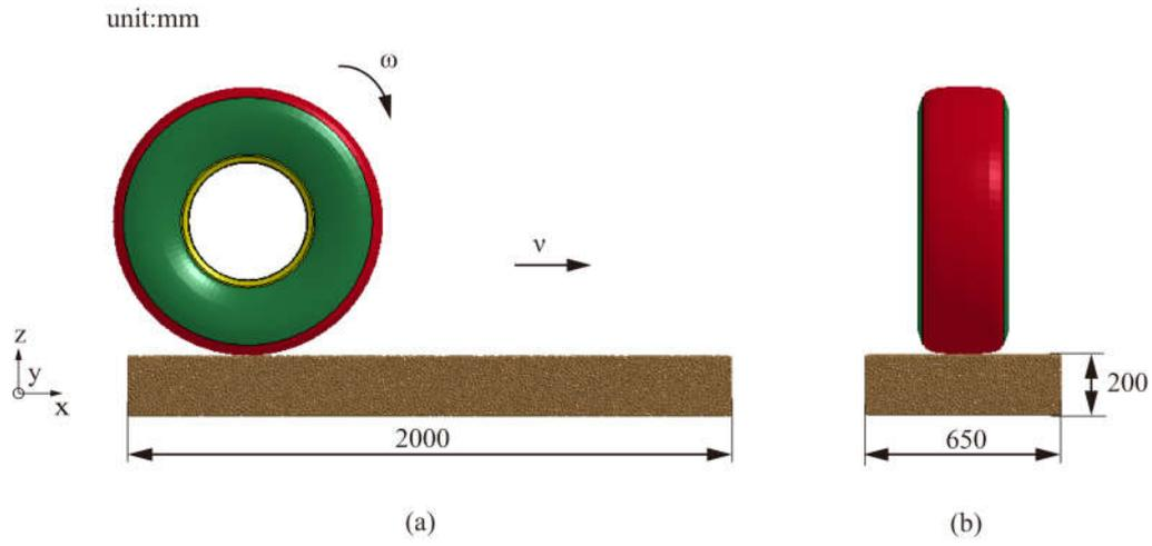
**Figure 5:** DEM-FEM model of tire-granular terrain interaction: (a) front view, (b) left view
