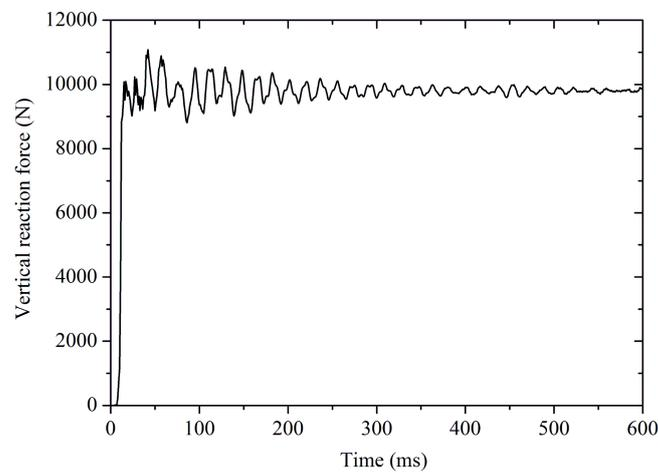
**Figure 7:** Time history of the vertical reaction force under the slip of 20%
