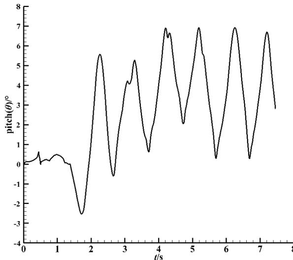
**Figure 11** The pitch response of the floating structure.
