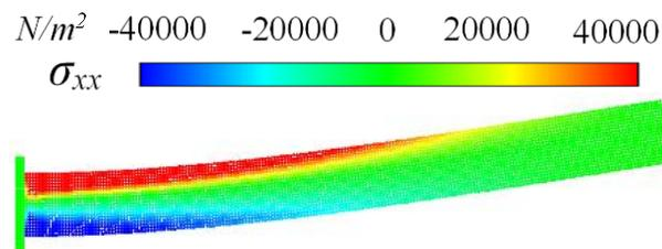
**Figure 5** The stress field at  $t=0.57$  s
