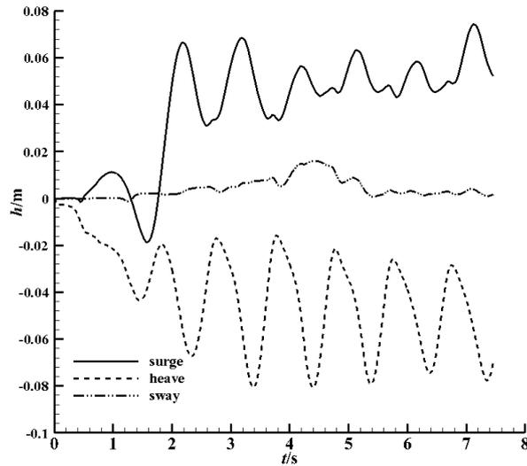
**Figure 10** The surge, heave and sway response of the floating structure.
