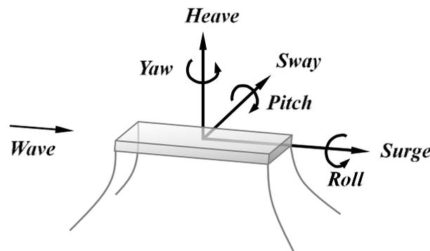
**Figure 7** Description of motion responses of floating structure.
