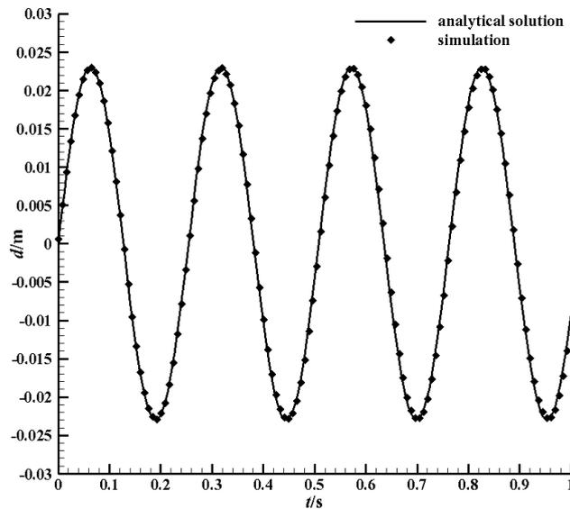
**Figure 4** The deflection at the free end of the cantilever beam
