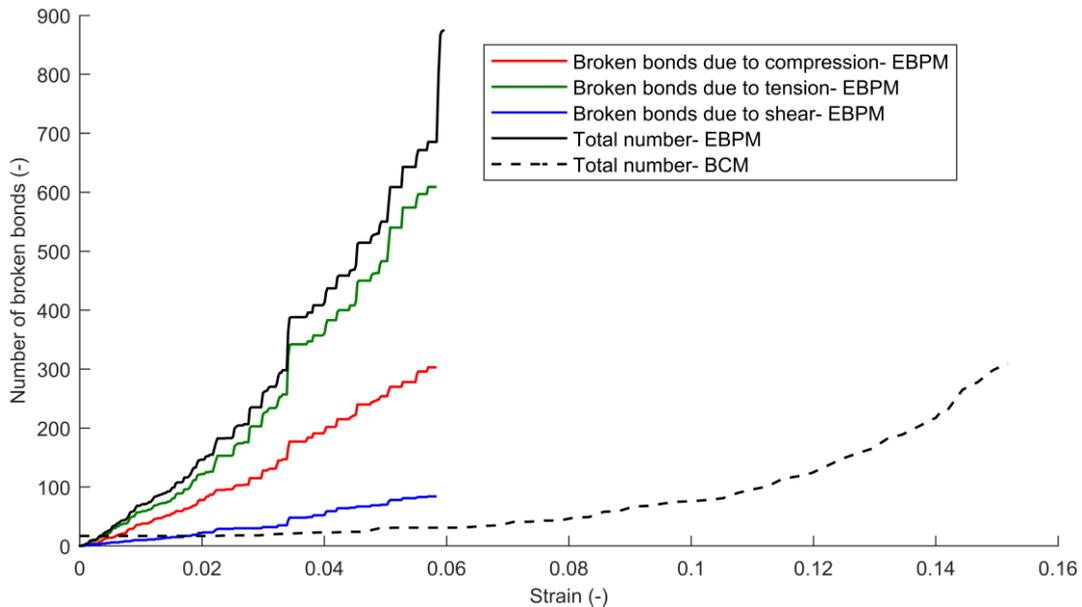
Figure 6: Number of broken bonds up to failure using BCM and EBPM models
