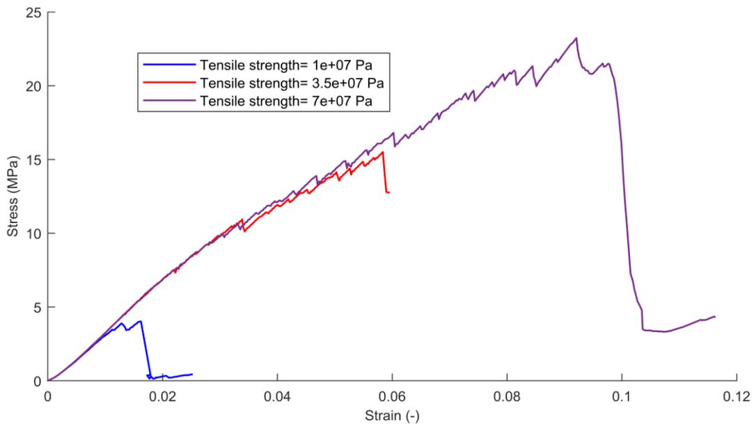
Figure 7: Effect of tensile strength on the stress-stain curve of EBPM
