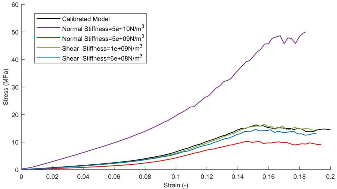
Figure 5: Effect of normal and shear stiffness of BCM on the stress-strain curve
