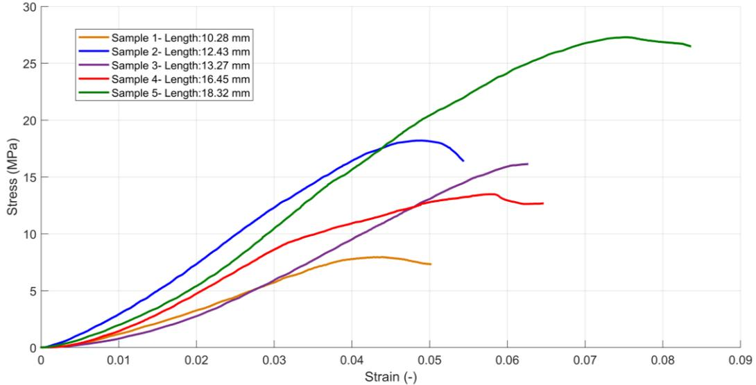
Figure 2: Experimental results of the uniaxial compression test with five different pellets
