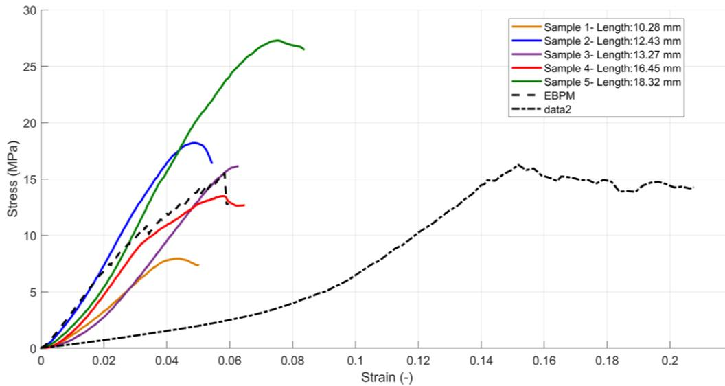
Figure 4: Stress-strain results of experimental and numerical methods
