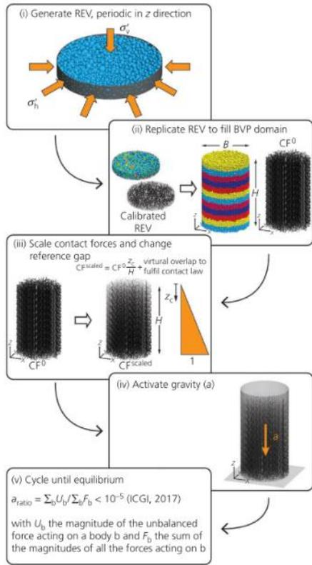
Figure 1: Flow chart outlining the steps to initialize a sample using the periodic cell replication method [10]
