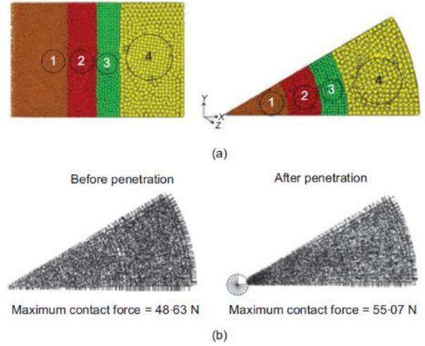
Figure 2: Example use of the particle refinement method a) particle scale locations. b) contact forces within the sample[11]
