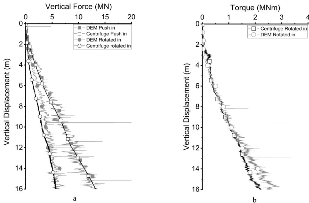
Figure 4: Geotechnical Centrifuge tests vs DEM for the installation of axially jacked and rotary jacked piles. a) Vertical force vs vertical displacement, b) Torque vs vertical displacement [12]
