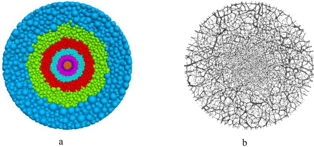
Figure 3: Example of a cell produced with varying scales. a) A layered soil using the dimensions from Table 2, b) Contact forces of the cell once isotropic consolidation has occurred
